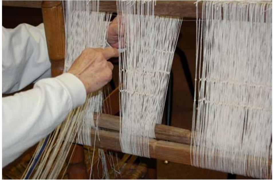
**Threading the heddle.** A heddle is a series of parallel wires or cords used to separate warp threads and make a path for the shuttle.
